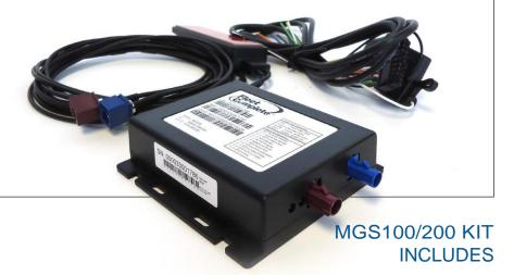
MGS Device Power Harness Covert Antenna (MGS200 only) 1 Blue Terminal Ring 4 Zipties
